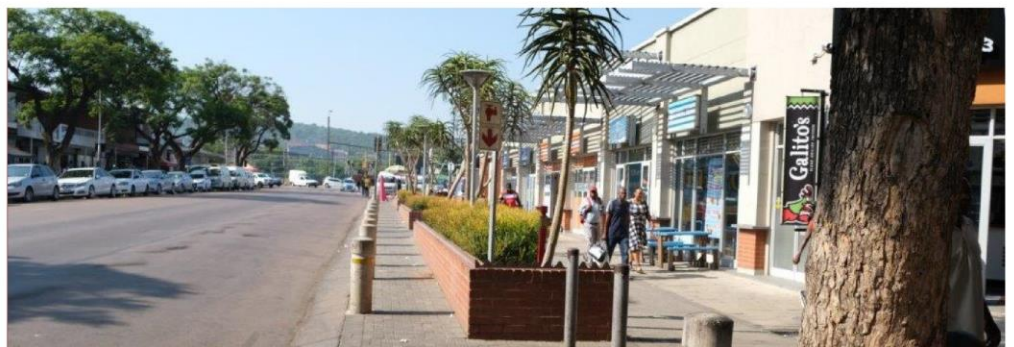
Bulb-outs in a parking lane can accommodate street furniture and amenities without compromising pedestrian mobility
