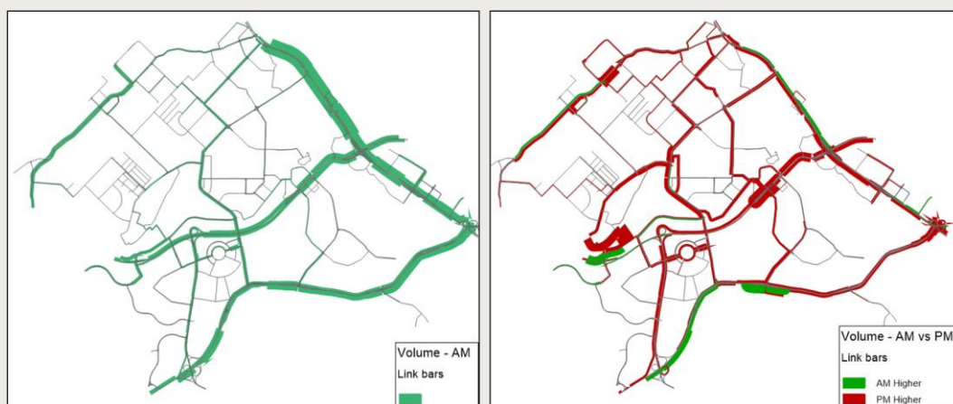
Transport Model applications – Highway mesoscopic vehicle flows
