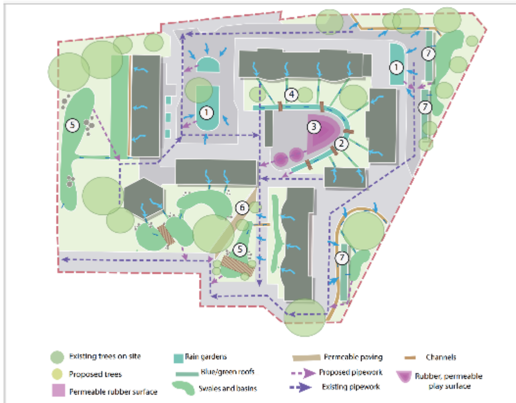
Reimagining rainwater in the social housing sector. Figure 2.10 - Concept for SuDS in social housing
