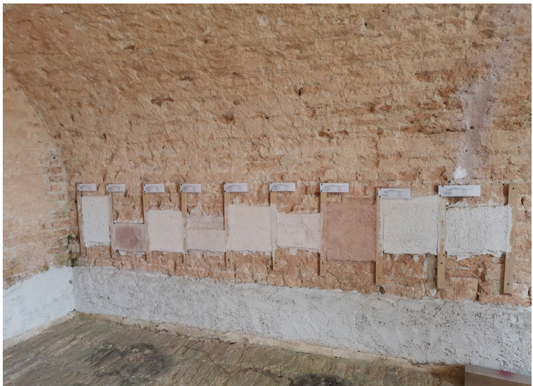
Plasterwork testing at Fort Cornwallis
